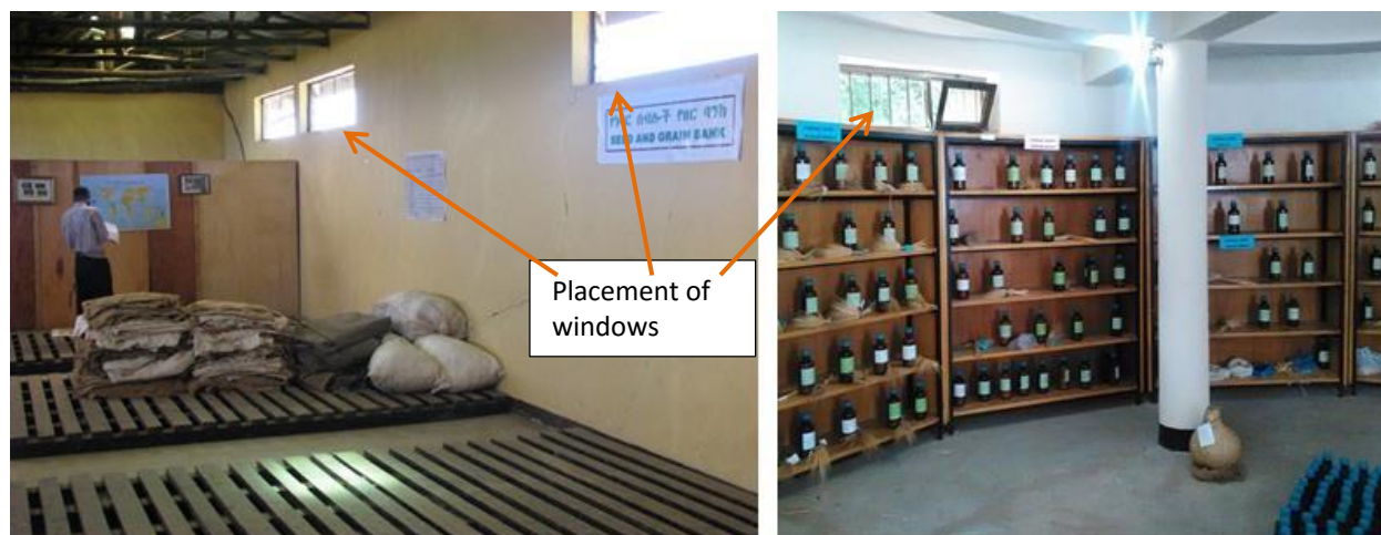
Fig. 6 Placement of windows of (L) a seed store and (R) germplasm unit for good air circulation
